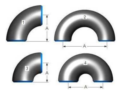
3D elbows as an example, are calculated with: 3(D) x 2(NPS) x 25.4
