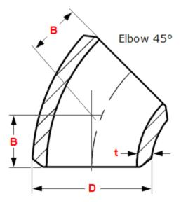
The radius of a 45° elbow is the same as the radius of the 90° LR (1½D). However, the center to face dimension is not equivalent to the radius as in 90° LR elbows. This is measured from each face to the point of intersection of the center lines perpendicular to each other, distances B on the image. This is due to the smaller degree of bend. Short radius 45° elbows are not available.
