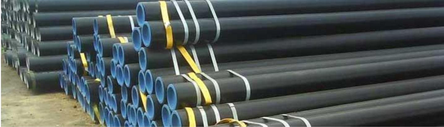
For a given NPS, the outside diameter stays constant and the wall thickness increases with larger schedule number. The inside diameter will depend upon the pipe wall thickness specified by the schedule number.
